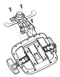
3B. Place the mechanism on the underside of the seat as shown, then reattach the bolts.
