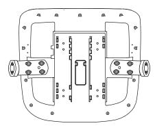
2B. Adjust the left and right arms to be symmetrical, then reattach the bolts to secure the arms.
